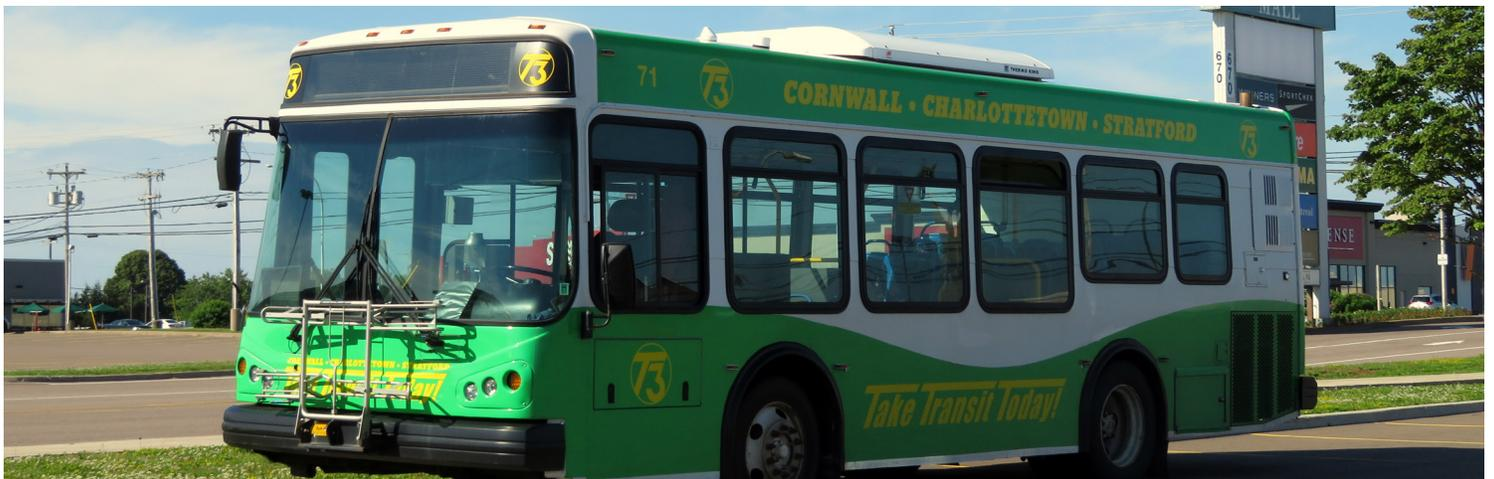
Figure 53: Small transit bus in Stratford, PEI. This bus model comes in lengths between 30' and 35'. (Photo Credit: Sean Marshall; CC BY-NC 2.0)
